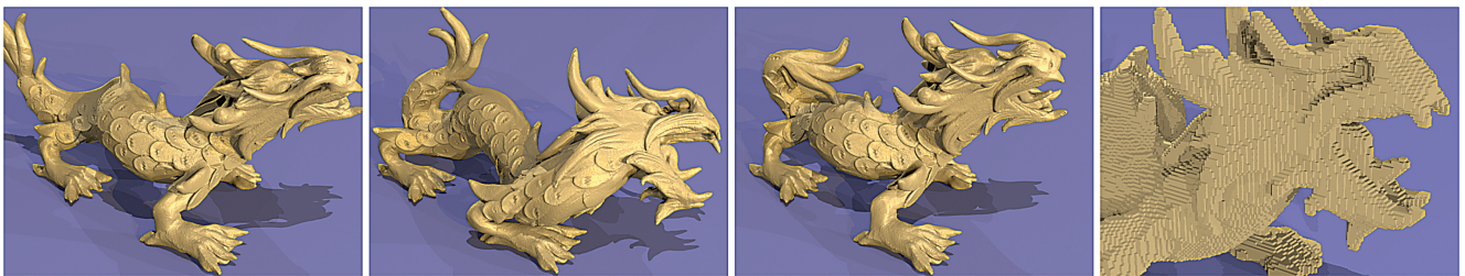
Fig. 27. Embedded animation of a deformable dragon shaking his head, using corotational linear elasticity and simulation of dynamics. The embedded surface contains 7.2M triangles, while the simulated embedding cage has 402K cells (close-up pictured on the right).
